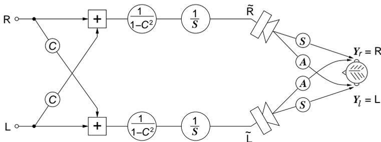
**Figure 6.** Crosstalk cancellation in head-related stereophonic sound field reproduction with two loudspeakers by prefiltering.  $S = S(\omega)$  and  $A = A(\omega)$  are the nearside and farside transfer functions, respectively, between loudspeakers and eardrums; circles to the left of the loudspeakers indicate filters with inscribed transfer functions,  $C = C(\omega) = -A(\omega)/S(\omega)$ .
