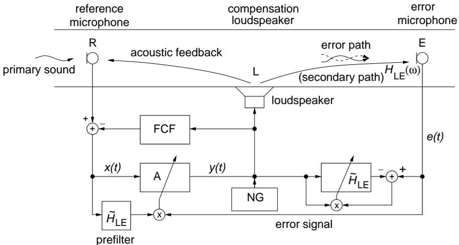
**Figure 3.** ANC in a duct by adaptive feedforward control with feedback cancellation and error path identification for the filtered-x LMS algorithm.
