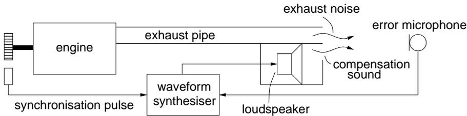
**Figure 5.** Active cancellation of (quasi)periodic noise by tracking control with sync input and waveform synthesis (after [51]).
